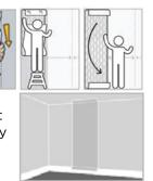
**IMPORTANT:** Do not pull or stretch the material during installation. Do not force, let gravity assist you. Or else patterns on the panels may not match perfectly. Work from the top and allow the wallpaper to fall naturally. For best results, have one person guide the paper at the top and along the seam, while another holds the opposite edge away from the wall until the seams are lined up.
